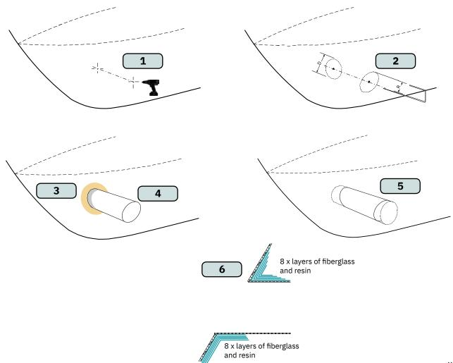
With tunnel installed and cast.
