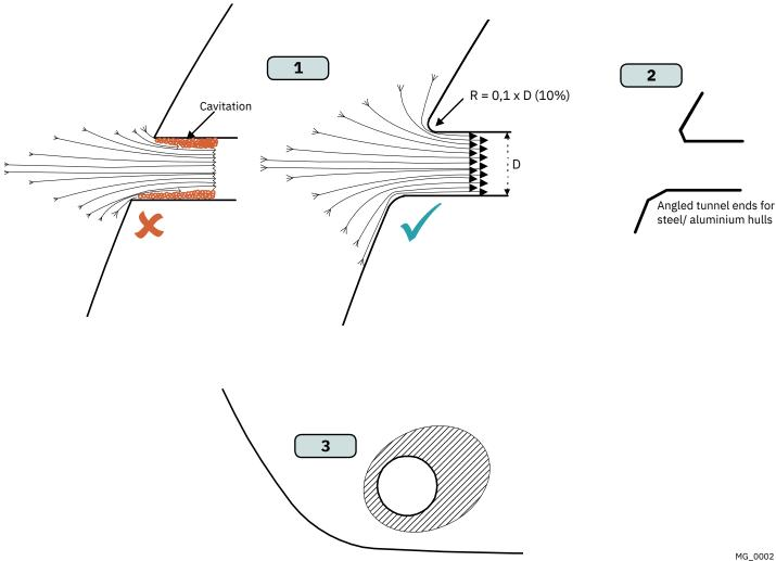
The following are only general instructions and do not explain in any way the details of fibreglass work. Problems caused by faulty installation of the tunnel, are the installers full responsibility. Seek a professional boat builder when modifying the hull.
