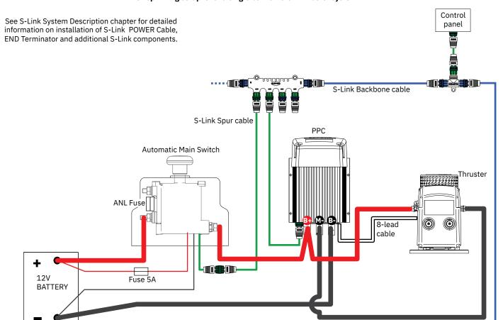
The top and bottom wiring setup is for a dual thruster system, For example bow and stern.
