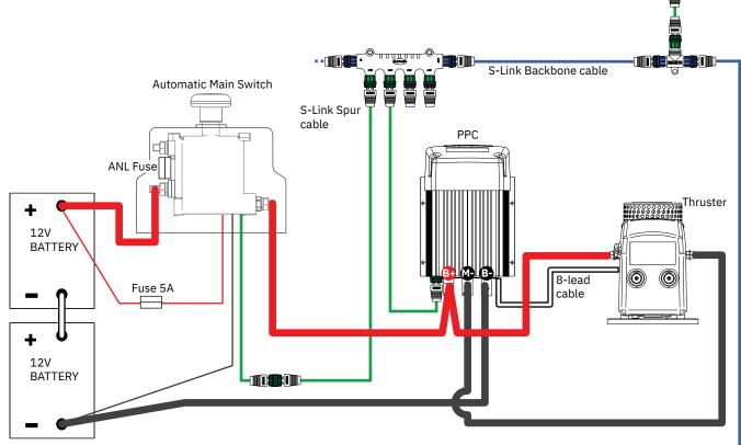
The top and bottom wiring setup is for a dual thruster system, For example bow and stern.
